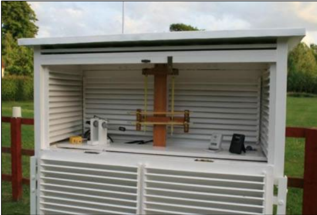
Figure 4 (below, right) – Conventional [large] Stevenson screen layout, showing maximum and minimum sheathed liquid-in-glass thermometers (mounted horizontally) together with the Vaisala HMP45C temperature and humidity sensor used in this comparison (grey cylinder, left of screen). This photograph was taken on 14 June 2009.
